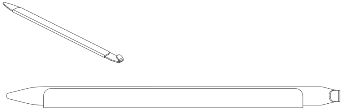
FIGURE 31 Optical transceiver (SFP+) extraction tool
